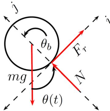
**Figure 4: Free Body Diagram of the Rotating Ball**
