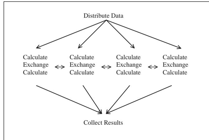
**Figure 1.5** Basic structure of a SPMD program.
